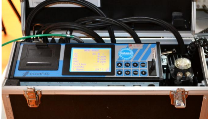
Figure 3-12: Portable gas analyzer.
