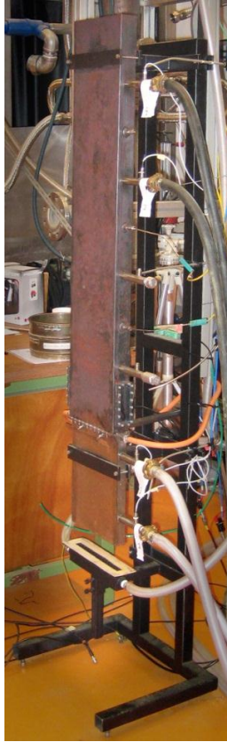
Figure 3-1: LIMOUSINE version 1 combustor.
